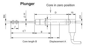
Fitted PVC cable, Ø6, optional length and termination
