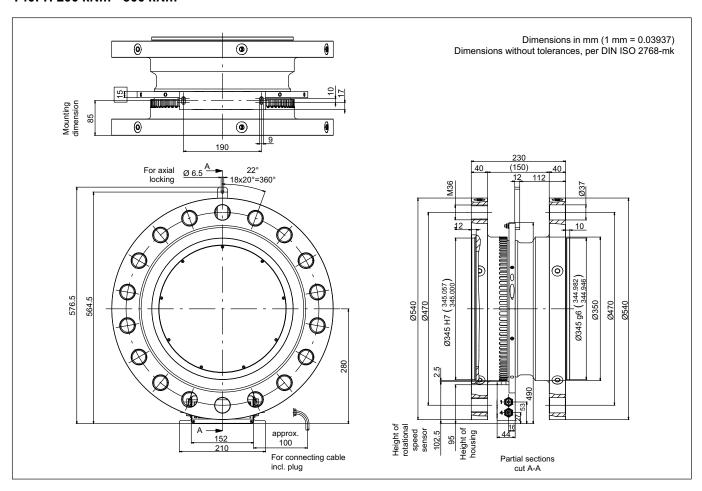
T40FH torque transducer (non-rotating), Option 4, Code PNJ T40FH 100 kNm - 150 kNm
